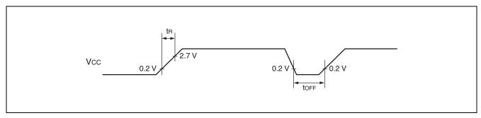
Note: If you change the power supply voltage too rapidly, a power-on reset may occur. We recommend that you start up smoothly by restraining voltages when changing the power supply voltage during operation, as shown in the figure below. Perform while not using the PLL clock. However, if voltage drops are within 1 V/s, you can operate while using the PLL clock.
